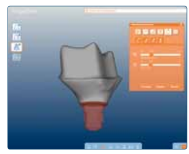
Two-piece Custom Abutment (ZrO 2 copings on a Ti base)
